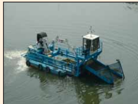
Deweeder Machine at WTP
