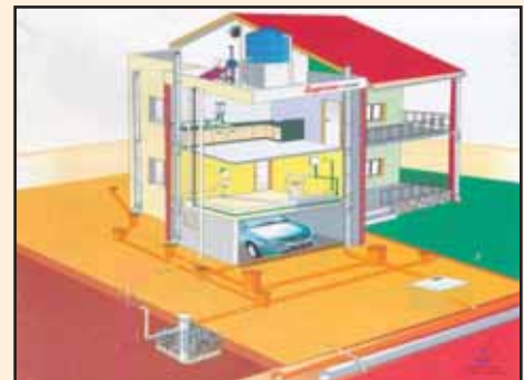
Underground and Overhead Tanks
